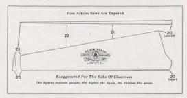
This grinding, exclusive with Silver Steel Saws, in connection with our method of cutting and setting the teeth insures Silver Steel Saws against binding or buckling.
