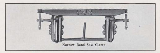
While this Clamp is designed primarily for filing Narrow Band Saws, it will be found an extremely convenient addition to any filing room equipment.
