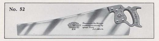
This saw is made for fine cabinet work, where a very smooth cut is essential. It is given an extra fine hard temper, so that the teeth may be sharpened to an extremely keen cutting edge. It is ground five gauges with an extra thin taper back, also slightly hollow, which gives it ample clearance. The teeth are sharpened to a needle point. It runs without set. Blade skew back, Atkins Silver Steel, high polish.
